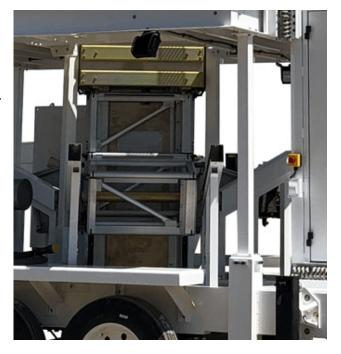
The three bales are mounted at 120-degree increments around the center of the tower, on a supporting trailer frame. Wound up on each bale is a hinged chain of varying length flat truss-like sections, nesting into a squared spiral. A set of hinges between each of the sections allows rotation for nesting.
