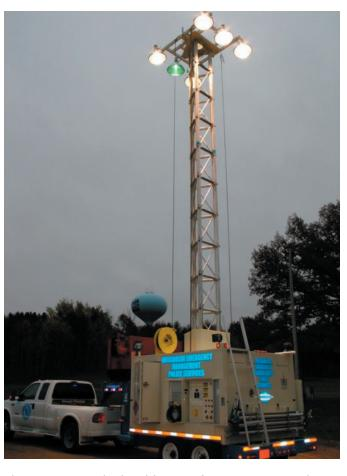
The <u>PTM-130</u> is deployable to 80 ft in 5 minutes and can lift 2,000 lbs. It has a compact trailer for portability, easy towing, quick setup, and stability.
