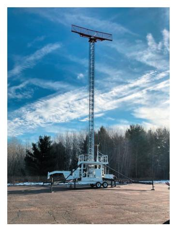
The **PTX-100** is deployable up to 120 ft in 8 minutes and can lift 2,000 lbs. It is designed with patented integrated outriggers and guy-wire connections to withstand winds over 100 mph.
